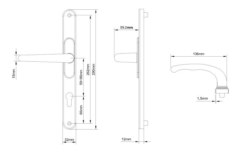
Technical Info Centres 59mm to 96mm (adjustable) Faceplate Width 32mm Screw Centres 262mm Spindle 8mm Pack Quantity 1 Pair Handle adjusted to your needs
