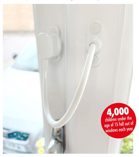
A small yet very effective and extremely affordable solution is the UAP keyless window restrictor. The keyless window restrictor has a 20cm long cable, which when installed correctly will limit the opening of the window to under 100mm. Not only will this prevent children from being able to fit through the gap, but it also allows enough air to circulate around a room.
