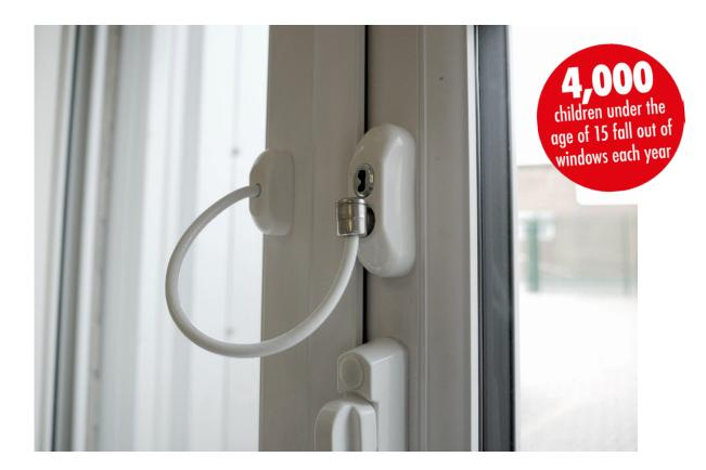
The window restrictor has a 20cm long cable, which when installed correctly will limit the opening of the window to under 100mm. Not only will this prevent children from being able to fit through the gap, but it also allows enough air to circulate around a room.
