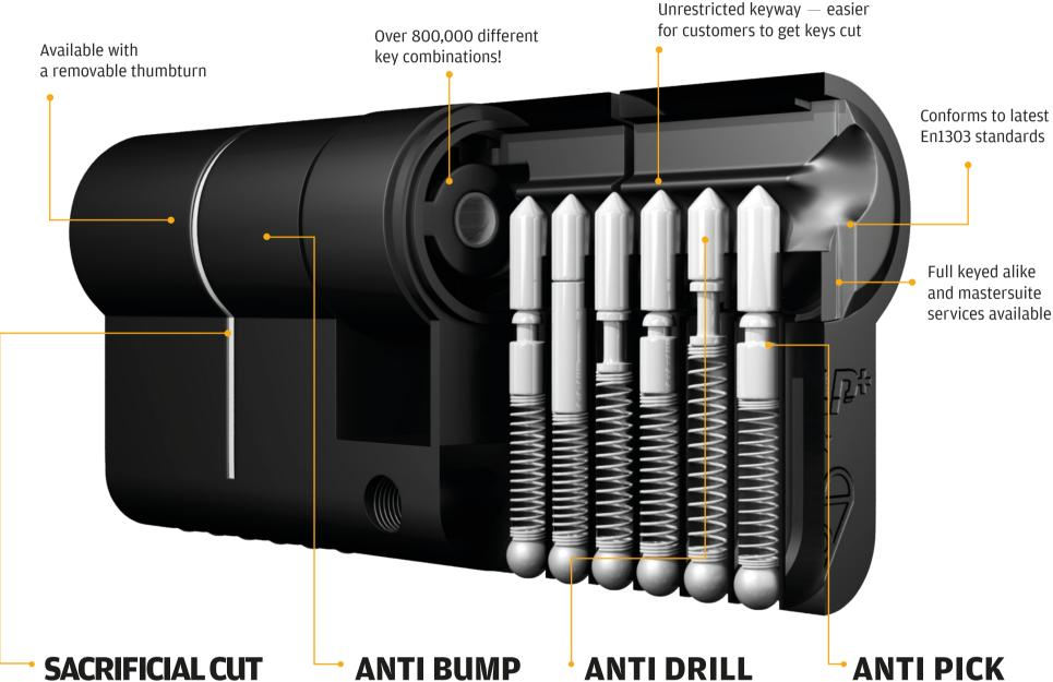
The cylinder has a Sacrificial cut on each side, so when force is applied to either end, the cylinder will break away to the sacrificial cut line only, leaving the remaining cylinder operational and the locking mechanism intact
